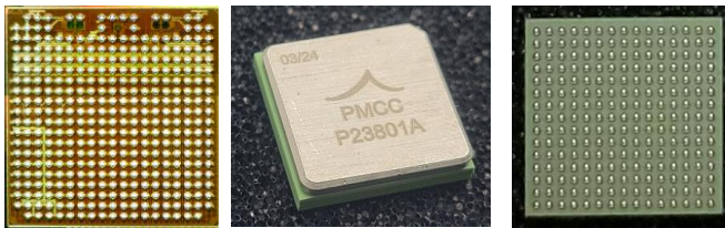
Figure 2. The chip photo and expected view of the BGA packaged ASIC part.
