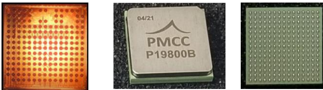
Figure 2. The ASIC chip and the BGA package.
