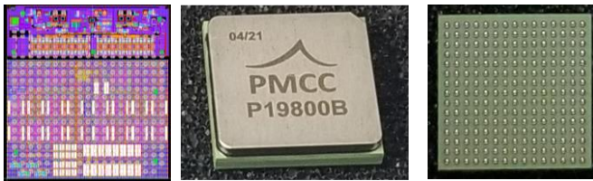
Figure 2. The view of the chip and expected view of the BGA package.
