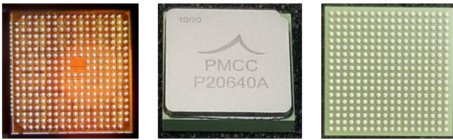
Figure 2. A chip photo (left), expected BGA package view (center) and the package ball array (right).
