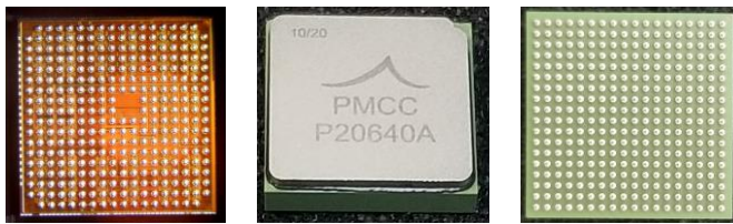
Figure 2. A Chip photo (left), BGA package (center) and the ball array (right).
