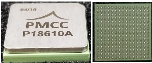
Figure 2. A BGA package for the ADC.
