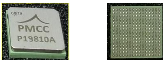
Figure 3. The ASIC in a BGA package.
