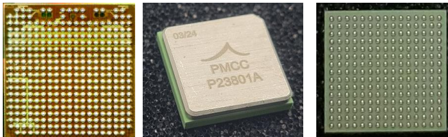
Figure 2. Chip photo and the BGA packaged ASIC part.
