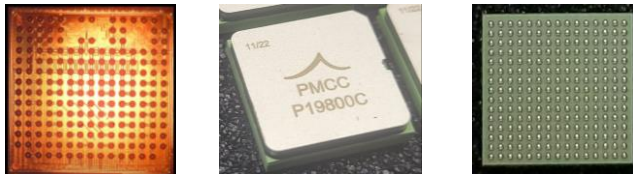
Figure 2. The ASIC chip and the BGA package.
