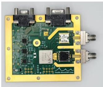
Figure 3. Evaluation board for the P19800B/C ASIC.
