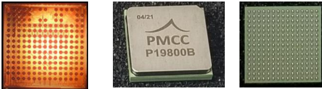
Figure 2. The ASIC chip and the BGA package.
