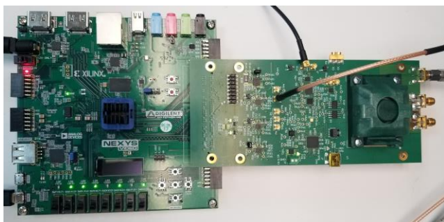
Figure 4. Evaluation board and test setup with socket.
