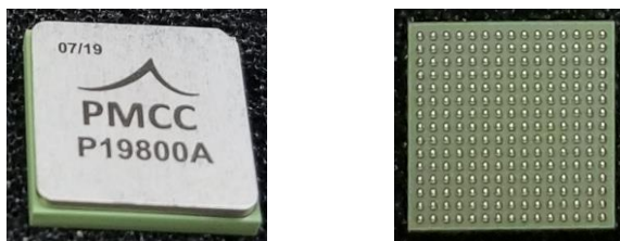
Figure 3. The ASIC in a BGA package.
